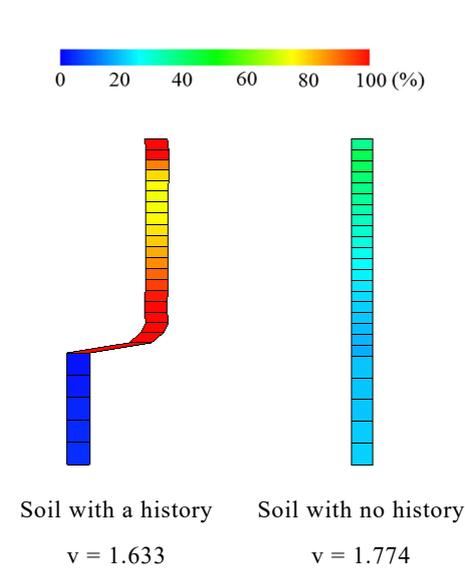
Fig.6 Excess pore water pressure distributions just after an earthquake
