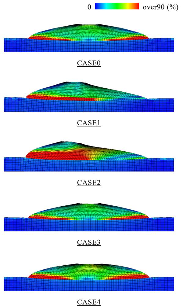
Fig. 2 Shear strain distributions just after earthquake
