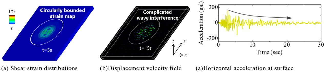
Fig. 3 1-phase elasticity analysis
