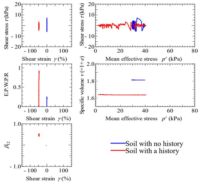
Fig. 7 Behaviors appearing in re-liquefaction factors
