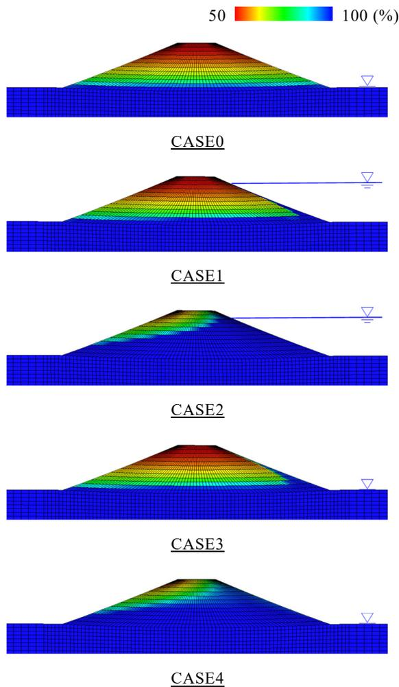
Fig. 1 Soil saturation degrees immediately before earthquake and river water levels
