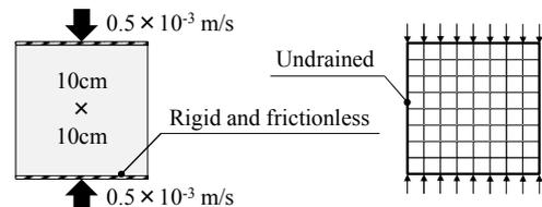
Figure 1. Undrained plane strain compression problem
