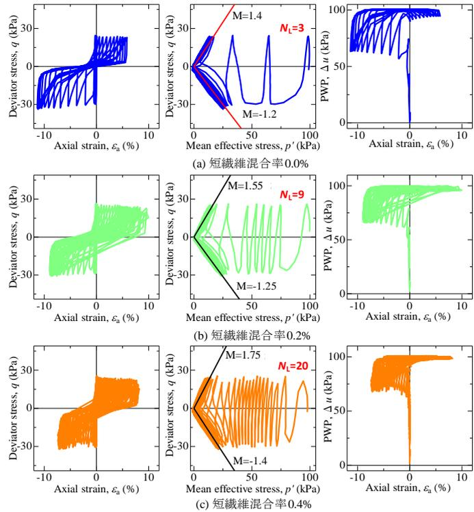
Fig. 2. Comparison of cyclic behavior of Mikawa sand N6 with different fiber contents ( $D_r=40\%$ ,  $p'_0=100\text{kPa}$ ,  $\text{CSR}=0.15$ )
