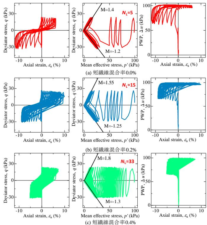
Fig. 3. Comparison of cyclic behavior of Mikawa sand R6 with different fiber contents ( $D_r=40\%$ ,  $p'_0=100\text{kPa}$ ,  $\text{CSR}=0.15$ )
