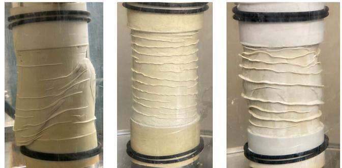
(a) 溶脱なし (b) 溶脱 60min (c) 溶脱 2day
