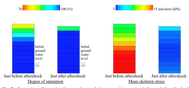
Fig. 7 - Comparison of saturation degree and mean skeleton stress between just before and after aftershock
