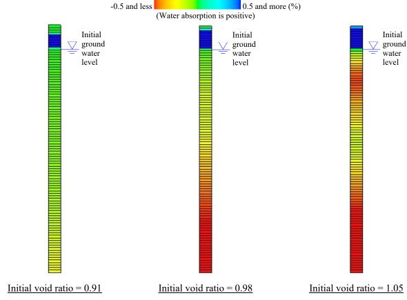
Fig. 9 – Comparison of water content change from the initial state in grounds with different initial void ratio, just after the earthquake
