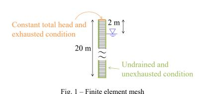
Fig. 1 – Finite element mesh
