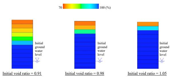
Fig. 8 – Comparison of saturation degree in grounds with different initial void ratio, just after the earthquake
