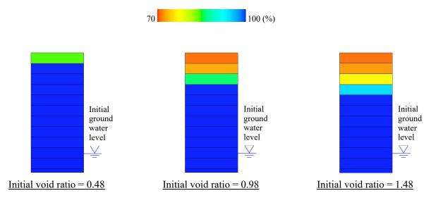
Fig. 10 – Comparison of saturation degree just after the earthquake among the grounds with unsaturated and elastic part above initial groundwater level, and with initial void ratio of 0.48, 0.98 and 1.48
