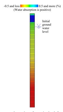
Fig. 5 – Water content change just after main shock from the initial state
