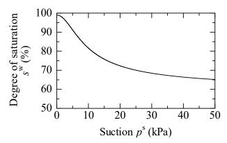
Fig. 2 – Soil water characteristic curve
