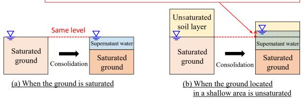
Fig. 6 – Schematic explanation of groundwater level rise mechanism
