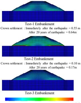
0 6 12 18 24 30(%) Fig. 8. Shear strain distribution 20 years after the earthquake.
