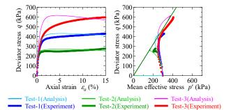
Fig. 5. Simulation of undrained shear tests. Table 2. Material constants.
