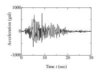
Fig. 7. Input seismic motion.
