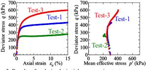
Fig. 3. Results of undrained triaxial compression test.
